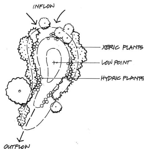
Depiction of typical bioretention area design illustrating shallow slopes, well drained soil profile and location of plant material along hydrologic gradient. Basins with large catchments should include an over drain or provide a spillway in case of high flow event, and underdrains can be used in areas with low conductivity soils.
