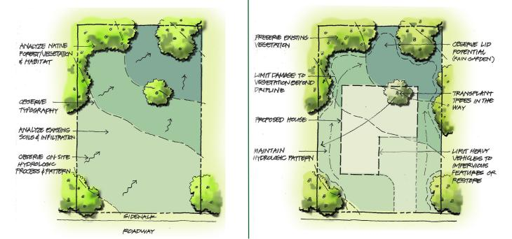
Diagram of site considerations before and after placement of house on site. Integrity of drainage pattern and canopy cover are maintained and soils are evaluated for placement of on-site LID practices such as a rain garden, permeable surfaces or exfiltration system.
