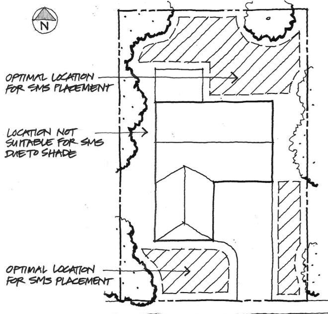
(Above left) Layout of irrigated areas showing optimal and unsuitable locations for sensor placement.
